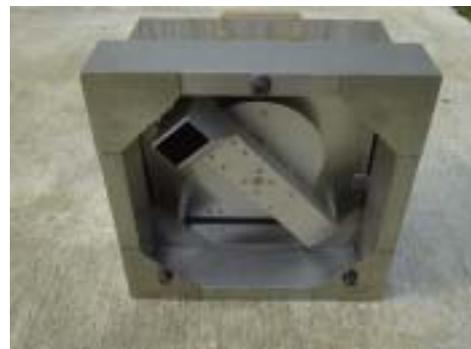
Picture 2 Laser Displacement Sensor of CTM
