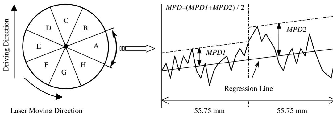
Fig.2 Calculation of MPD from CTM Measurements
