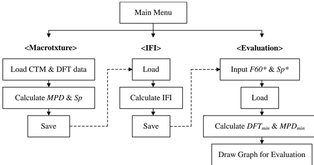
Fig. 7 Flow Diagram of the Software
